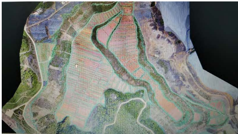
Figure 3. UAV remote sensing slope analysis diagram of Dexing Copper Mine 300 dumpsite ecological restoration project (1:1000)
