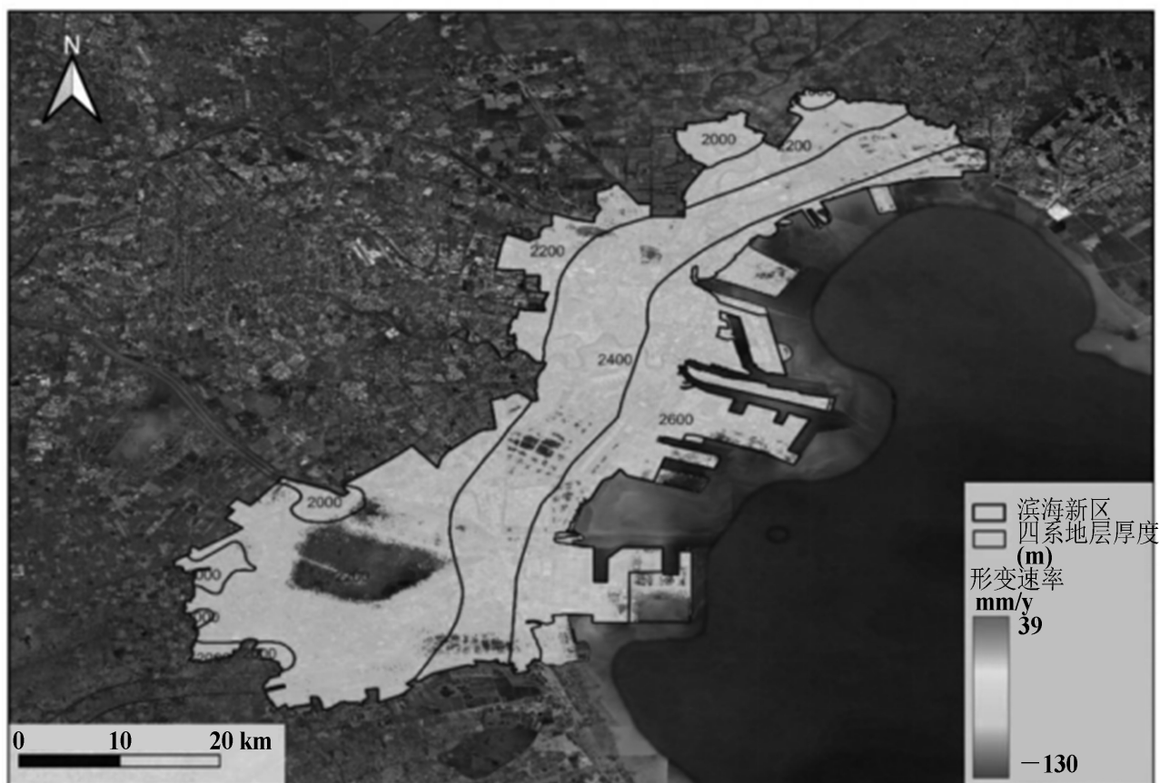
Figure 4. Spatial overlay of ground settlement results and quaternary strata thickness
