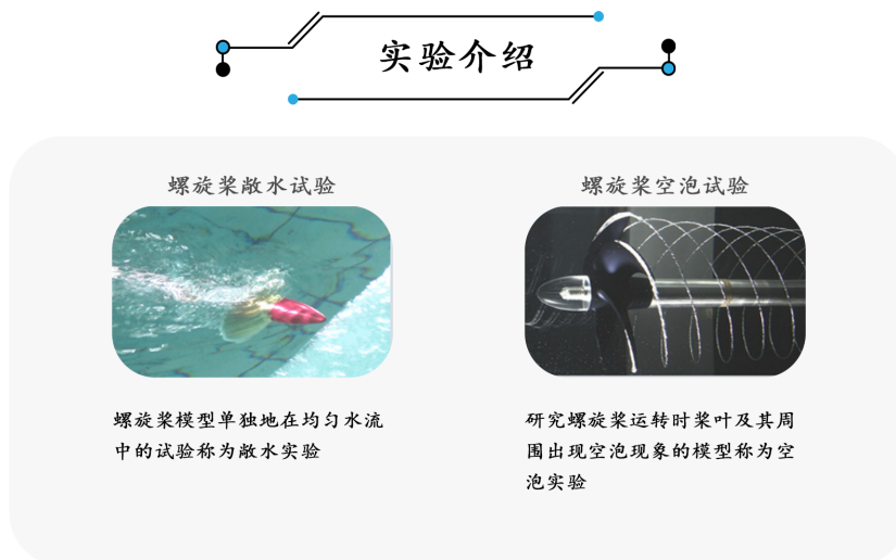
Figure 3. Selection interface for propeller open-water test and cavitation test 图 3. 螺旋桨敞水试验和空泡试验选择界面
