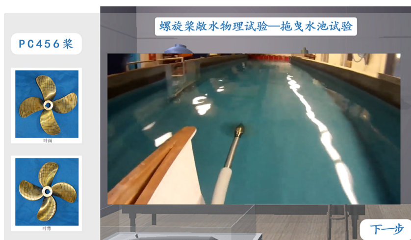
Figure 6. Propeller open water test interface
