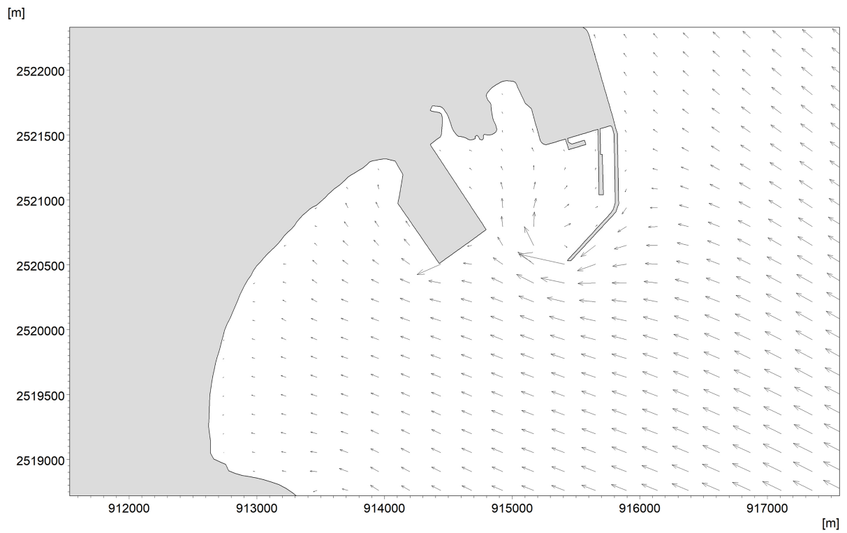
Figure 7. After the project, the tidal surge and rapid flow field in the sea area 图 7. 工程后海域大潮涨急流场
