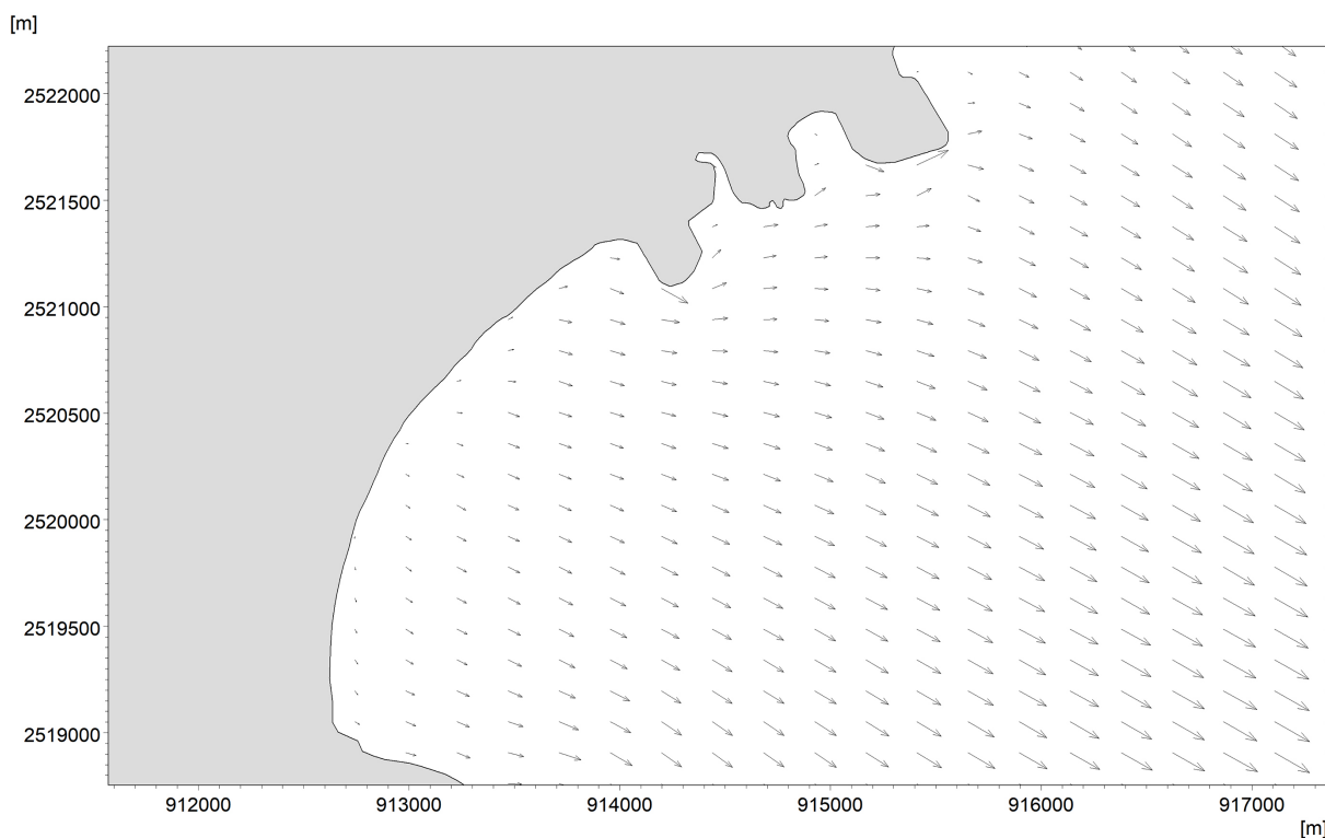
Figure 6. Before the project, the rapid flow field of high tide and low tide in the sea area 图 6. 工程前海域大潮落急流场
