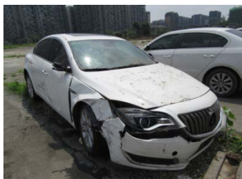
Figure 3. Damage to the right front 图 3. 轿车右前部损坏情况
