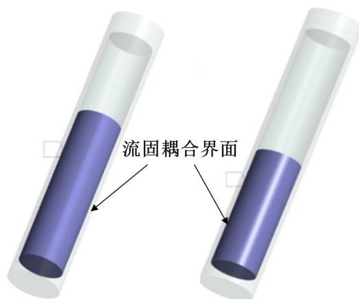
Figure 5. Definition of fluid-solid coupling interface in the accumulator barrel
