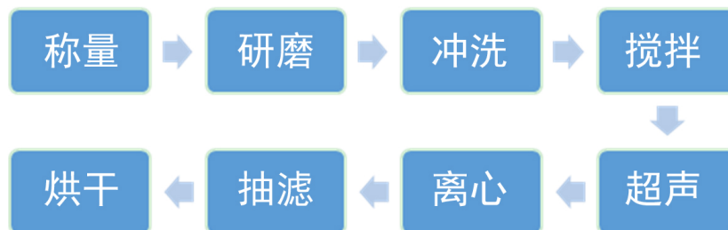
Figure 1. Preparation process of carbon nanotube buckypaper 图 1. 碳纳米纸制备流程
