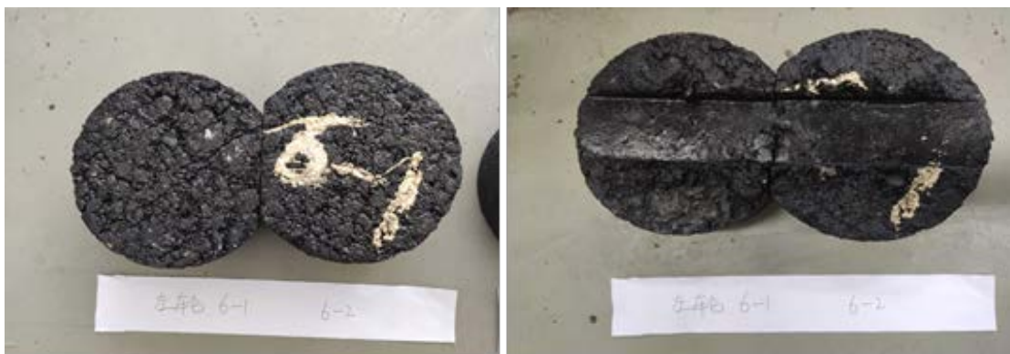
Figure 6. Surface changes of core samples before and after the Hamburg rutting test 图 6. 汉堡车辙试验前后芯样表面变化
