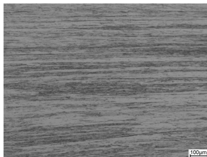
Figure 2. Metallographic photos of molybdenum-lanthanum alloy sheets in the rolling direction 图 2. 钼镧板轧向照金相片
