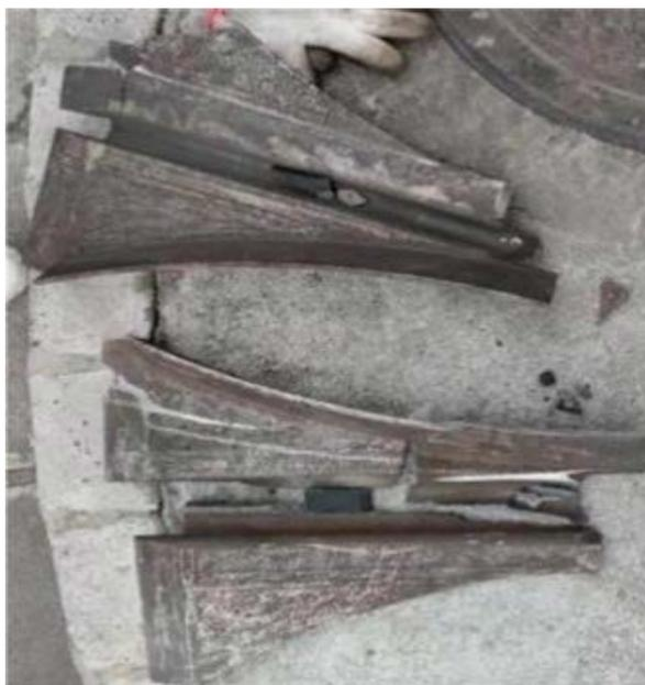
Figure 8. Damage diagram of HT250 re-railer
