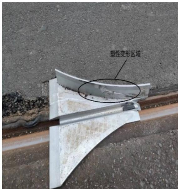
Figure 9. 40Cr re-railer after re-railing
