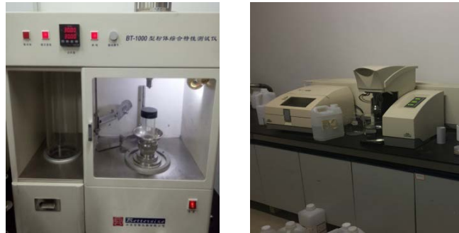
Figure 3 Physical property detection of powder comprehensive performance tester (left) laser particle size analyzer (right)
