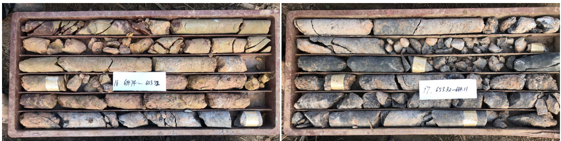
Figure 3. 2021-F1-Shui1 Hole F1 fault zone core photo (650.60~664.11 m)
