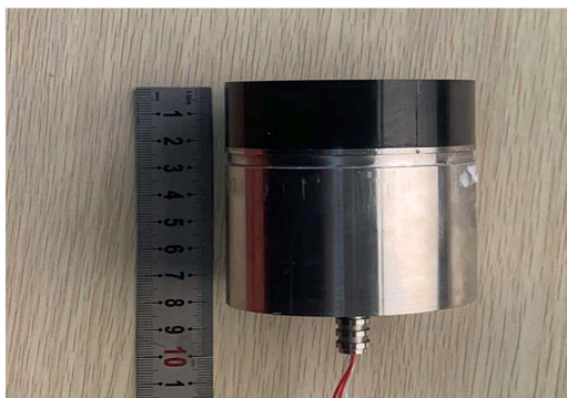
Figure 1. Relaxor ferroelectric single crystal/piezoelectric ceramic hybrid excitation transducer 图 1. 弛豫铁电单晶/压电陶瓷混合激励换能器
