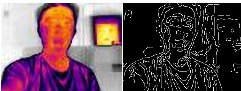
Figure 14. Portrait image after 4 times reconstruction (left) and after Canny operation (right) 图 14. 人像经过 4 倍重建(左)与 Canny 算子处理后(右)
