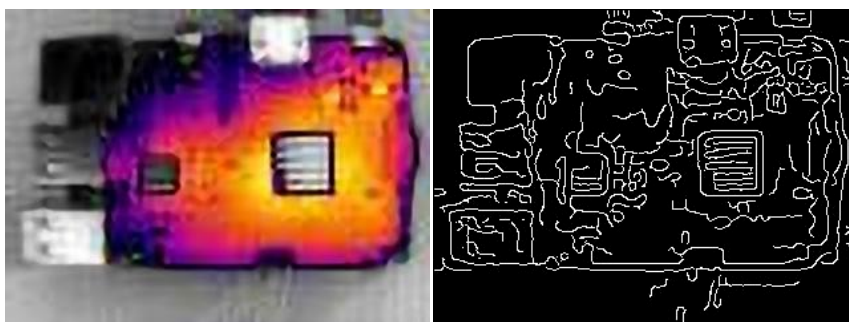
Figure 16. Raspberry Pi 3 image after 4 times reconstruction (left) and Canny operation (right)
