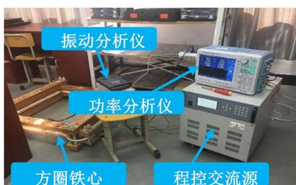
Figure 17. Diagram of vibration measurement experiment
