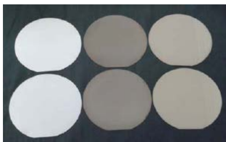
Figure 4. The physical drawing of ordinary piezoelectric wafers and reduction wafers
