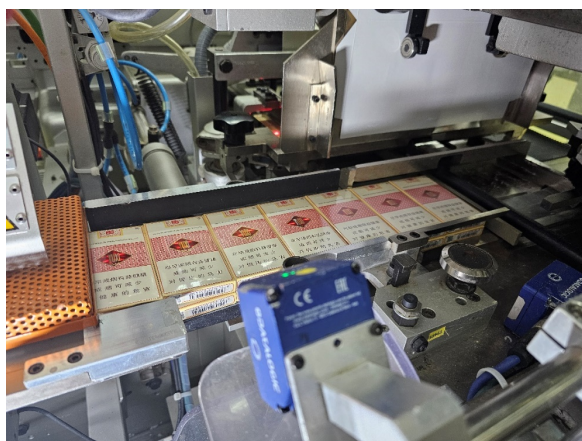
Figure 1. Physical map of the tobacco bale propulsion passage 图1. 烟包进烟通道
