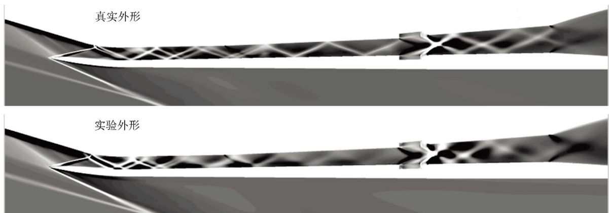
Figure 7. Schlieren photograph of inlet symmetry plane
