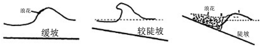
Figure 2. The shape of wave at different slope 图 2. 不同坡度下的波浪形态
