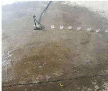
Figure 9. Wetted body of senqi micro-nozzle after nozzle modification
