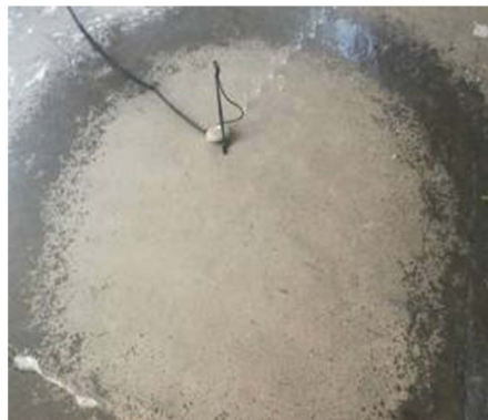
Figure 8. Wetted body of senqi micro-nozzle 图8. 原森芪微喷头的湿润体
