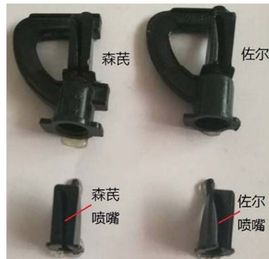
Figure 3. Nozzle of senqi and zuer micro-nozzle
