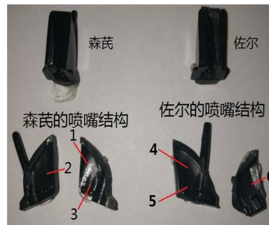
Figure 4. Internal structure of senqi and zuer nozzles
