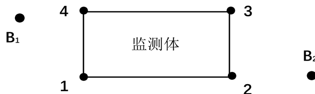
Figure 1. Sketch map of sedimentation observation with benchmark 图 1. 有基准沉降观测网络示意图
