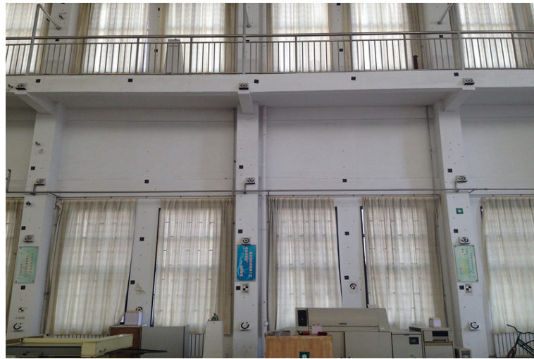
Figure 1. The experimental wall with a reflective marker 图 1. 粘贴反光标志的实验墙
