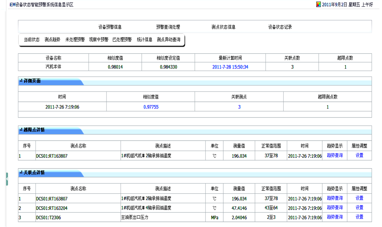
Figure 2. Turbine proper off-limit measuring points and association measuring points 图 2. 汽机本体的越限测点和关联测点
