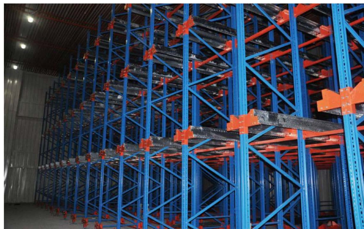
Figure 3. The racking system of a pallet shuttle AS/RS 图 3. “穿梭式”仓储货架系统示意图
