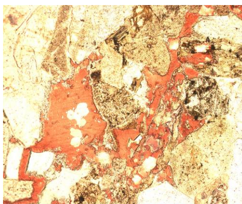
Figure 7. Well Gao 41, 888.5 m, calcite metasomatism, orthogonal light, \times 200
