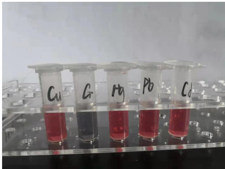
Figure 8. Reactions of ammonium Metatungstate-AuNPs with different heavy metal ions
